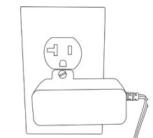
Route and secure the power lead, then plug the DC connector into the GDZW7-LR. The status LED on the GDZW7-LR will illuminate solid green upon powerup, if already added to the Z-Wave network.
